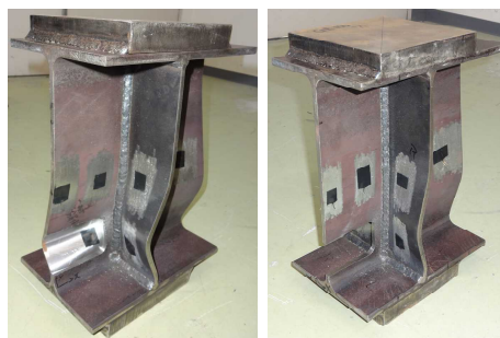
Compression test on main girder end specimen with partial volume loss
