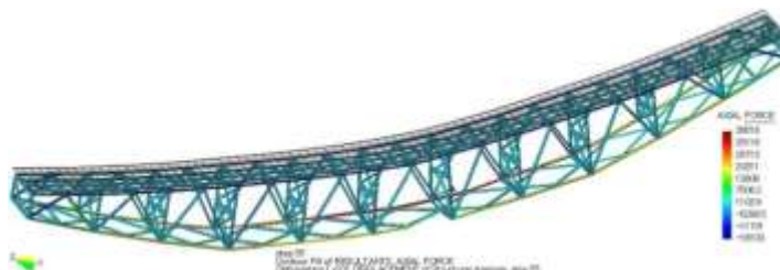
Numerical verification of redundancy against collapse of the steel truss bridge caused by fracture of a member
